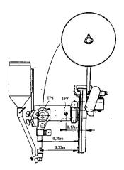
L<sub>max</sub> of the vertical slide is 0,1 m and of the horizontal slide 0,4 m. The deflection of the contact device due to the deformation of the slide profiles of the slides can be estimated as follows:
