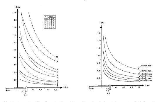
Vertical mounting. Bending of slide profile. Standing horizontal mounting. Twisting of slide profile.
