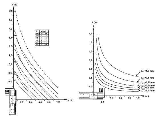
Lying horizontal mounting. Change of the centre of gravity in the Y-direction. The slide profile bends.
